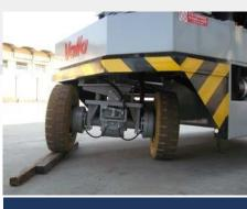
Rear steering with hydraulic cylinder between chassis and traction group for great performance also on not flat surfaces
