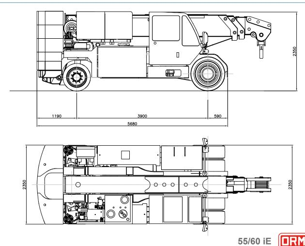
The steering radius is as limited as possible because the crane rotates on itself thanks to two slewing bearing units positioned in the rear wheels; the hydro-pneumatic suspensions system assures a perfect distribution of the load on the rear wheels.
